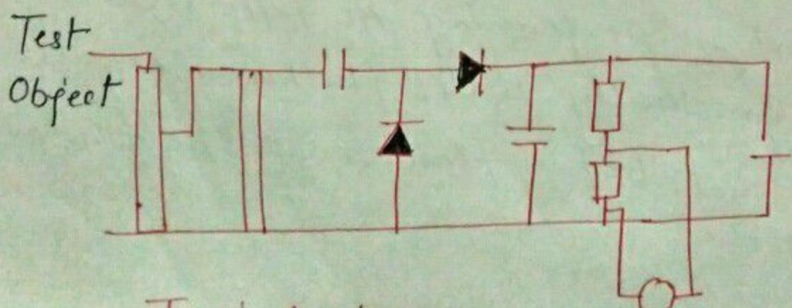
Typical doubling circuit for DC tests
