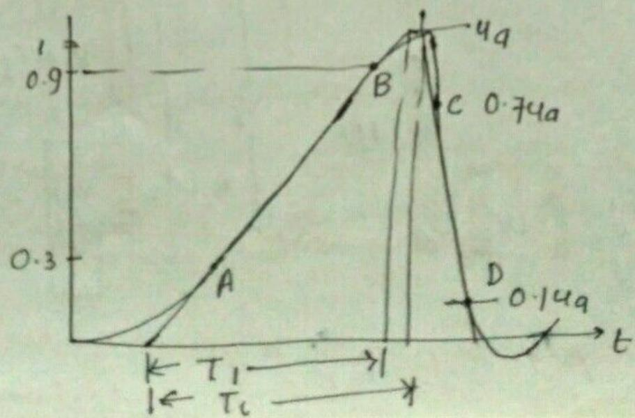
Example of lightning impulse voltages with aperiodic waveform
